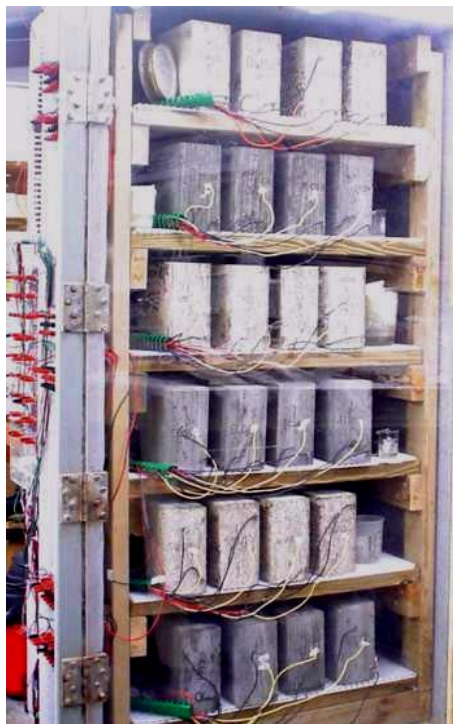
Figure 6 - The 95% RH test chamber.
