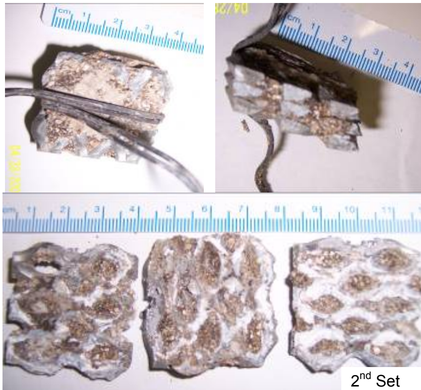
Figure 3 - Type W anode specimens. Zinc alloy anode appearance after embedded mortar was stripped. Top 1st set. Bottom 2nd set. (Mortar only partially stripped).
