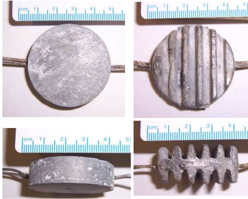
Figure 2 - Type C anode specimens. Zinc alloy anode appearance after embedded mortar was stripped; otherwise as-received. Left, 1st set; Right, 2nd set.
